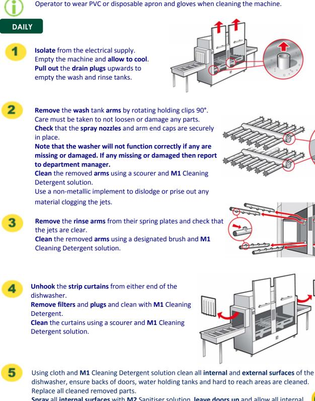
Spray all internal surfaces with M2 Sanitiser solution, leave doors up and allow all internal surfaces to air dry.
