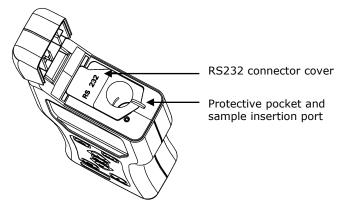
For details on the RS232/USB connector and protective pocket, refer to sections  $\underline{5.6}$  and  $\underline{6.1}$  respectively.
