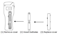
When the batteries are inserted correctly, the unit will automatically turn on and enter the clock set-up mode. (see section 3.8).
