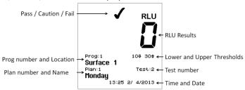
**TIP**: A failed test result  $\chi$  can be selected for retesting by pressing the  $\bigcirc$  button, followed by the  $\bigcirc$  button to select the Program location (see section 4.2).
