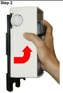
Attach the system to the bracket and slide it down...
