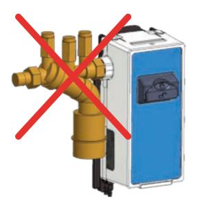
Do not install the BA valve directly at the inlet of the system to avoid inlet fitting breakage due to valve weight
