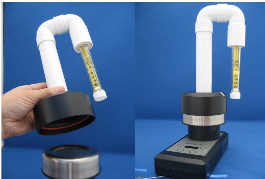
Figure 3: Fitting validation rig to the MB1/MB2
