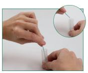
3. Return the swab to the extraction buffer and break off into the tube.
