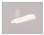
4. Place the device on a flat surface and allow the test to develop for 5 minutes.
