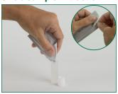
1. Tear or cut Type 8 extraction buffer sachet and fold corner to create a funnel. Add to a sample tube.
