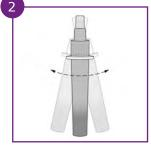
Add **0.2 mL** liquid sample (or rinse water), or weigh in **0.2 g** of homogenized sample into the extraction tube. Fill with **extraction buffer** to the level shown in the picture. Close the tube with the cap and vigorously shake by hand for **1 minute**. You can squeeze the tube to help suspend the sample.
