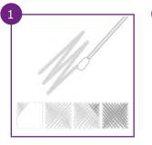
Fill one extraction tube with extraction buffer up to the neck of the tube (see step 1 for solid/liquid samples). Wet a swab by dipping it into the buffer. Wipe an area of 5 x 5 cm using side-to-side movements, rotating the swab tip as you go. Place the swab into the extraction tube and carefully break off the end at the pre-scored point. Close the tube with a cap and shake vigorously for **1 minute**.
