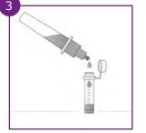
Remove the smaller cap to open the dropper tip and transfer **6 drops (200 \muL)** into an incubation vial. Close the lid of the vial.
