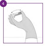
Shake the incubation vial vigorously by hand for **15 seconds**. Make sure that the liquid comes into contact with the lid of the vial.
