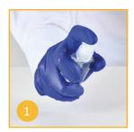
Moisten the sampling area with a sufficient amount of deionized or distilled water.
