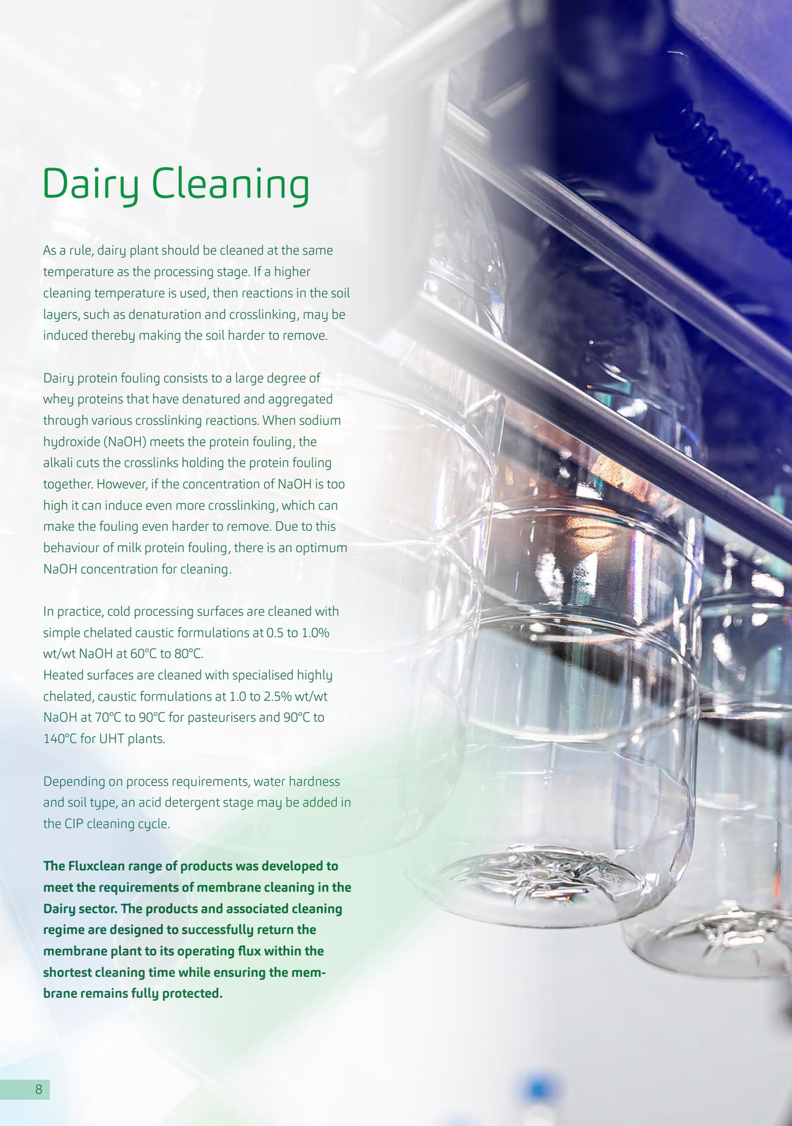
As a rule, dairy plant should be cleaned at the same temperature as the processing stage. If a higher cleaning temperature is used, then reactions in the soil layers, such as denaturation and crosslinking, may be induced thereby making the soil harder to remove.
