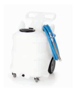
Vessel Capacity: Approximately 95 litres Air Supply Required Pressure 4 to 6 bar (60 to 85 psi) Flow 10 m3/h (150 litres/min) Air Inlet Connection: 3/8" hosetail
