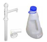
A drum pump with a push pull action made from polypropylene. There are two sizes available to fit 25 or 200 litre containers. As an optional safety measure a container can be purchased separately, which when screwed directly on to the outlet of either pump prevents accidental spillage of the chemical whilst decanting.
